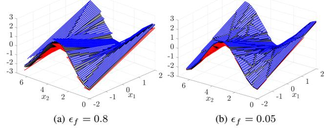
Fig. 3: Piecewise affine abstraction of  $x_1 \cos(x_2)$  using Method II (Theorem 2) with different desired accuracies.
